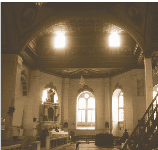
The sophisticated design of the church can be seen in many places, especially in the space at the crossing. The “arms” of the transept are unique, with walls diagonal to the nave. This configuration is also seen in the churches of Inabanga (Bohol) and Mandaue (Cebu).
