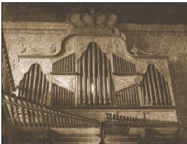
Fig.1 The façade of the Bamboo Organ with clearly two sets of trumpets (32 on the left side, 29 on the right) reflecting the divided keyboard. Of the bamboo pipes, only the pipes of the three towers are speaking, or a total of (7 \times 3 =) 21 .
